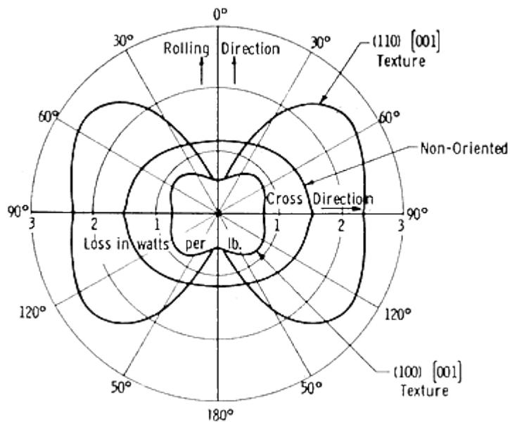
This diagram shows the magnetization behaviour of GOSS and non-GOSS strip relative to rolling direction The I-E Core
